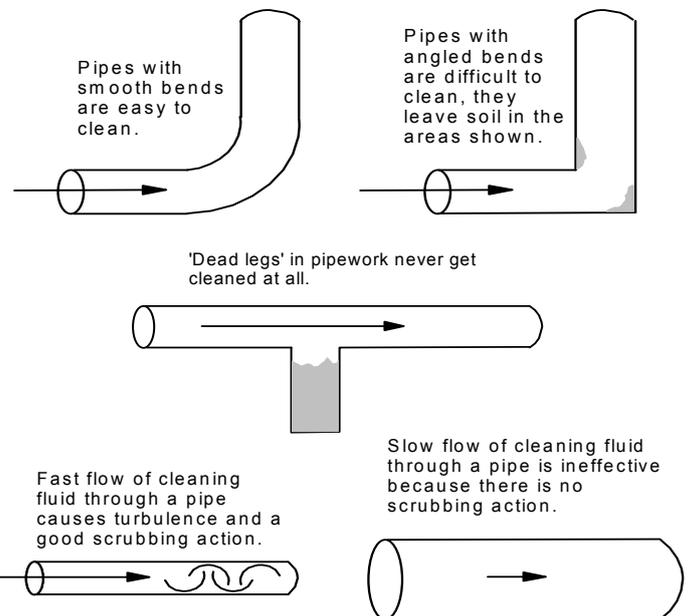
A pipe circuit for CIP should consist of pipes of the same diameter, otherwise the flow in the larger diameter pipework will be too slow.
