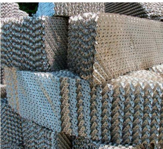
Figure 4: Structured packing segments prior to installation. Note the complex packing pattern, which maximises contact area
