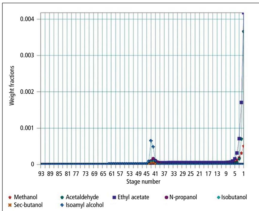
**Figure 7: Congener profile in a column. Fusel oils accumulate in the middle, while heads partition to the top of the column. Generated via SCDS model with ChemCAD**
