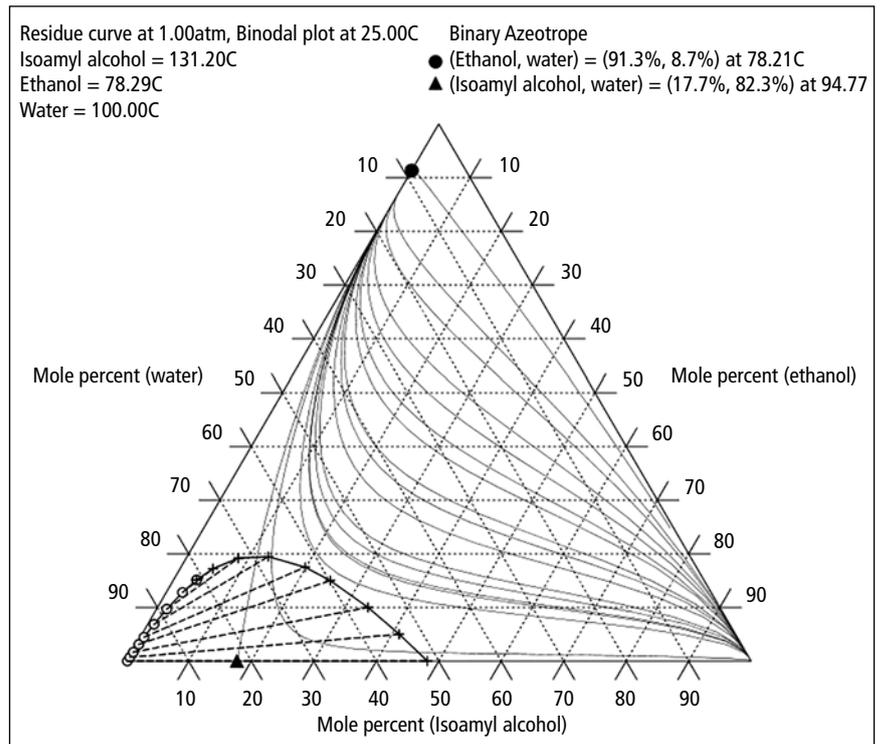
Figure 6: Residue curve between water, ethanol, and isoamyl alcohol via NRTL model on ChemCAD. Note the existence of two liquid phases in the absence of ethanol. This phenomenon can cause two-phase formation on column, and is exploited in the fusel oil decanter
