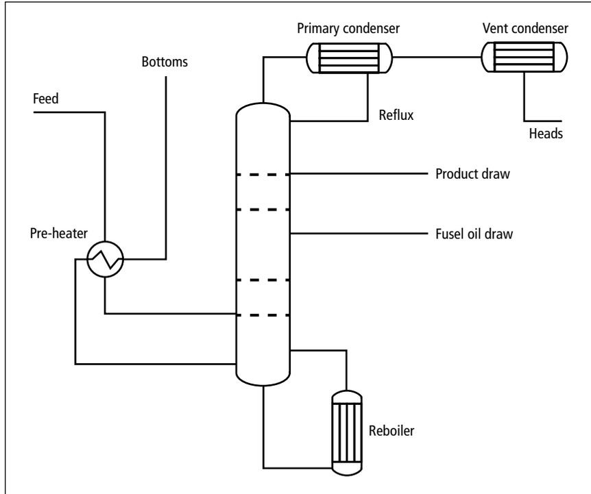
Figure 4: Simplified process flow diagram of a spirits distillation column
