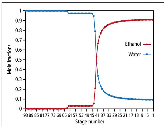
Figure 3: Typical ethanol/water profile along a brandy column, generated via ChemCAD SCDS model
