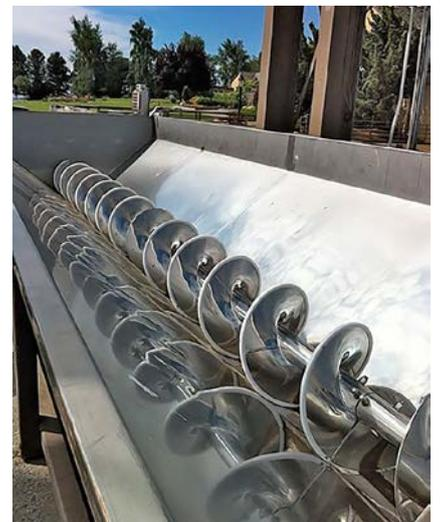
**Figure 1: A screw conveyor for handling grapes**
