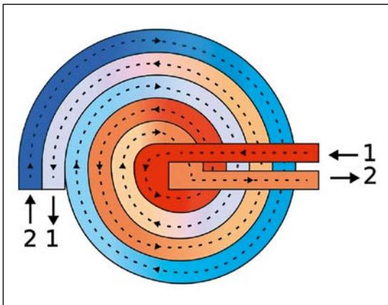
Figure 5: Flow patterns in spiral heat exchangers promote good heat transfer (due to counter-current operation) and resist fouling well
