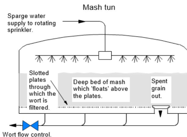
The traditional mash tun is a simple but effective system involving only one vessel for both the mash conversion and wort separation processes. It gives good quality wort but has a slow turn round time and is less efficient for extracting and transferring the enzymes, which are required to continue their activities in the washback.
