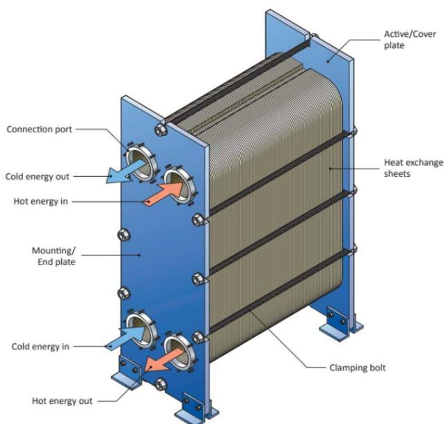
Figure 2 A plate heat exchanger.
