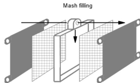
2. When the filter is full, wort drains from the mash into the plate on one side of the frame (the wort plate) and down
