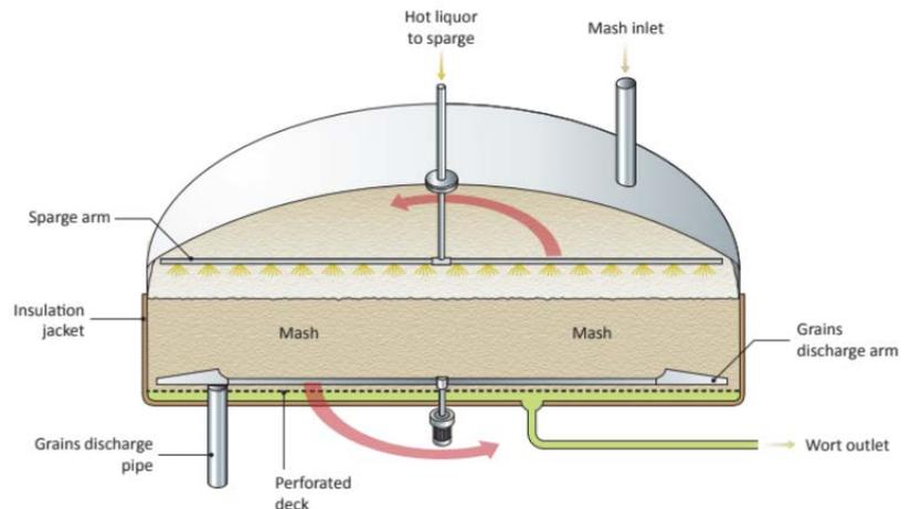
Figure 1 A 'mash tun', a combined mashing and separation vessel
