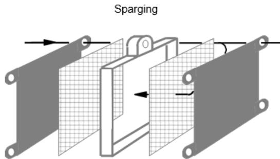
The spent grain is dropped from the filter at the end of the cycle when the filter is opened.
