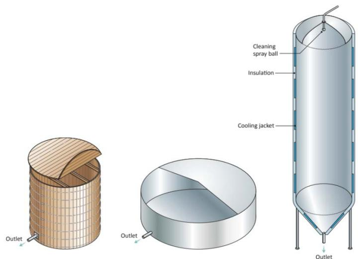
Figure 5 A traditional washback, flat-bottomed ferementer and cylindrical-conical fermentation vessel
