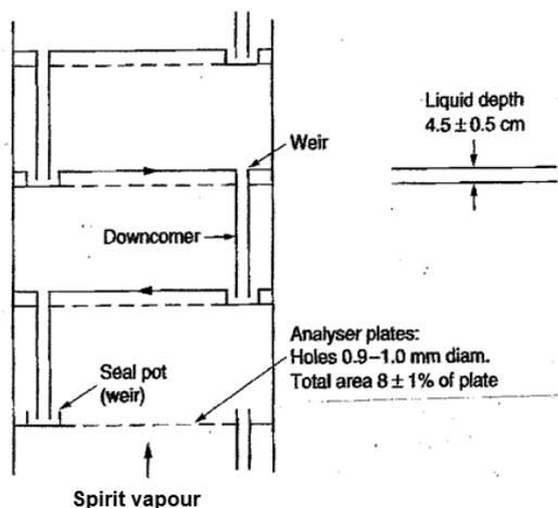
Figure 3 Flow across sieve plates between downcomer pipes.
