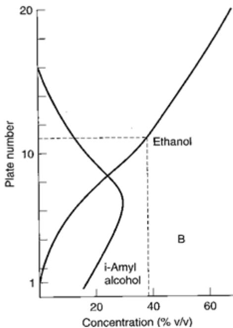
Figure 12 Effect of amyl alcohol concentration: restricted fractionation by high amyl alcohol concentration.
