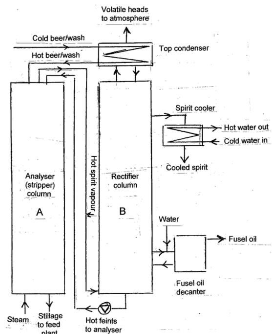
Figure 2 Continuous distillation of white rum or grain whisky.
