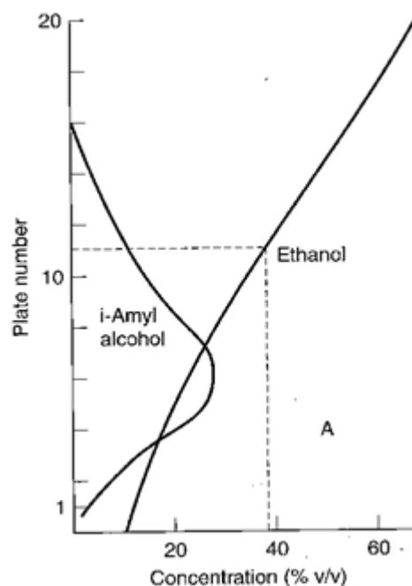
Figure 11 Effect of amyl alcohol concentration: normal operation of the lower section of the rectifier
