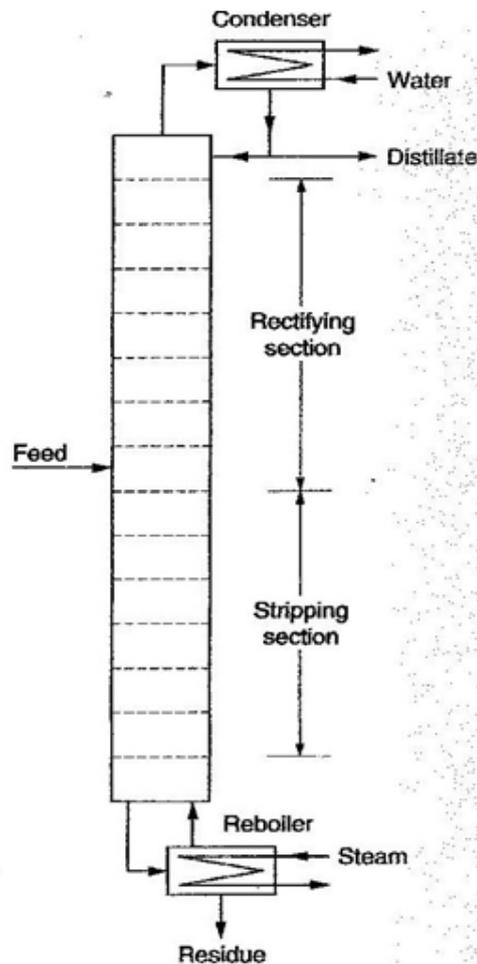
Figure 1 Simple distillation column.
