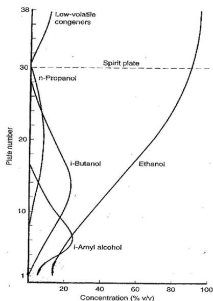
Figure 9 Congener profile in the rectifier column.
