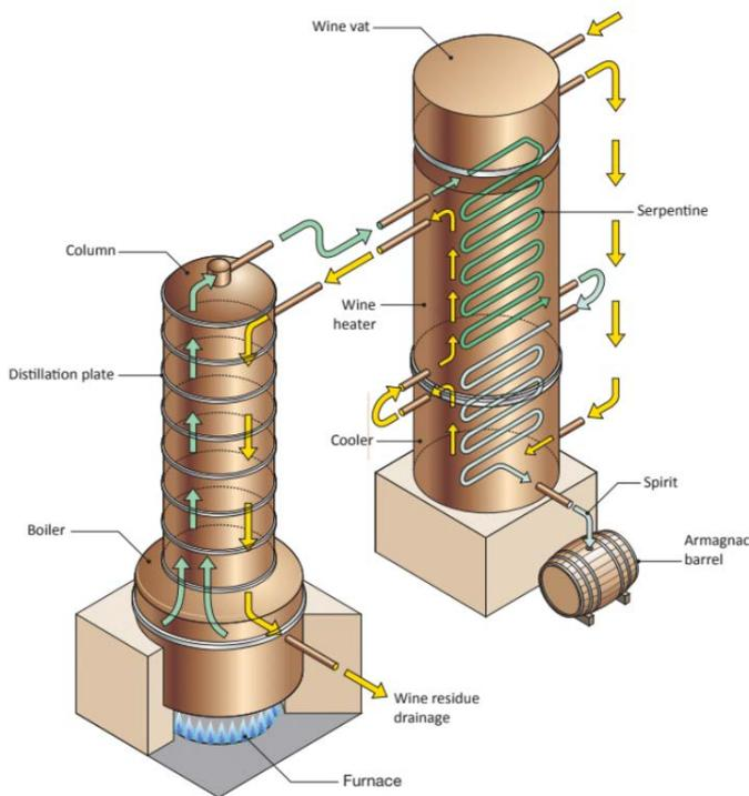
Figure 4 Column still for Armagnac production.
