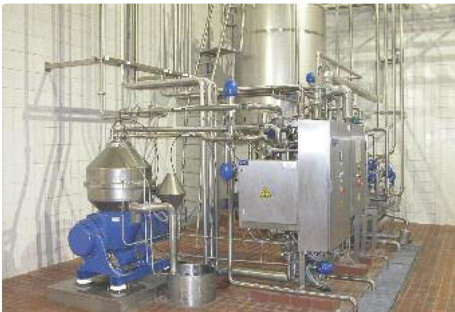
**Figure 6: Alfa Laval BRUX 510 continuous discharge separator module.**
