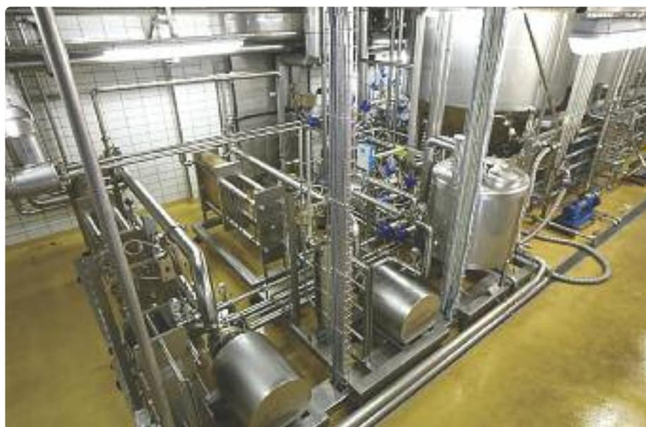
Figure 8: Alfa Laval cross-flow system for beer recovery installed at the Monchengladbach Brewery, features purpose-designed Alfa Laval microfiltration membranes, mounted in the Alfa Laval M39H plate-and-frame module.
