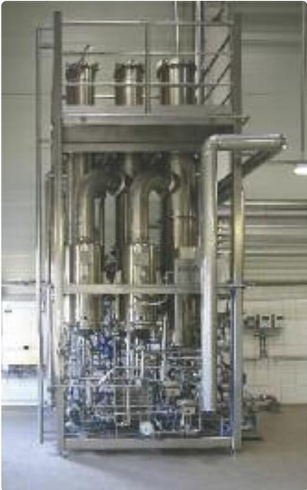
**Figure 3: Falling-film evaporation plant for the dealcoholisation of beer.**
