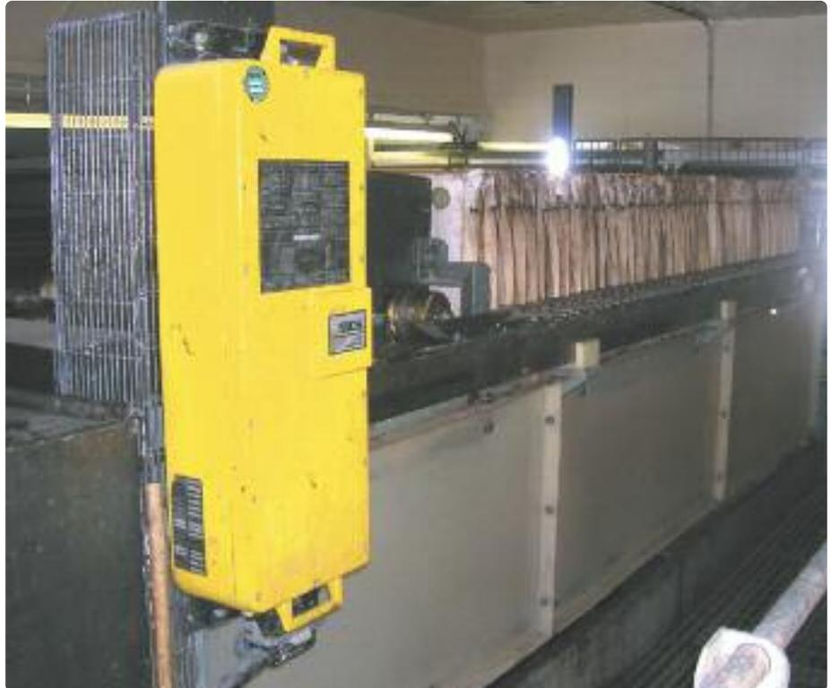
**Figure 1: A one tonne yeast press in a British brewery with polypropylene plates and frames installed in the 1980s.**
